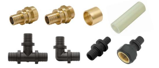
Tight connections without O-rings in the KAN-therm Push System are obtained by means of sliding the brass ring onto the fitting and pipe. The connections do not require any additional sealing, such as Teflon tape or tow. Manifolds and installation cabinets are a supplementation to the system.
